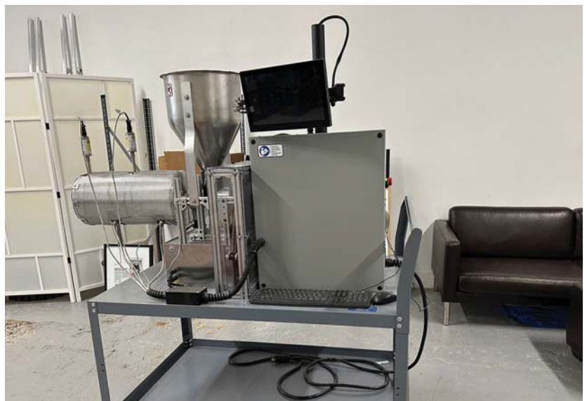
Redetec's MixFlow system builds on traditional extrusion processes. The proprietary solution separates the screw and the feed auger from the plastic and offers significant benefits in energy efficiency. Machine Design
