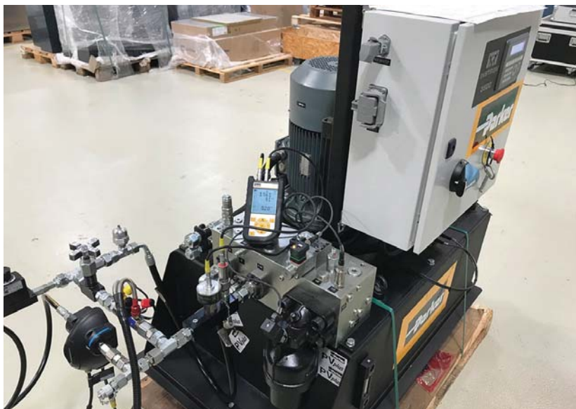
Use of maintenance tools like Parker Hannifin's SensoControl enables maintenance issues in hydraulic systems to be detected early before expensive downtime issues occur. Parker Hannifin Quick Coupling Division
