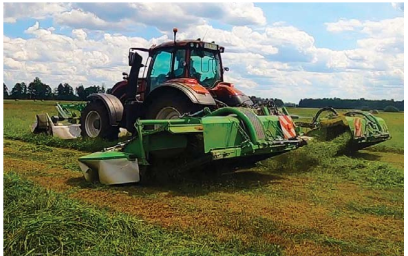
With the new electronic system developed by HydraForce, it was possible to receive ISOBUS certification which ensures the SaMASZ disc mower will work seamlessly with various models of agricultural tractors, ISOBUS terminals and other external equipment. Images courtesy of HydraForce
