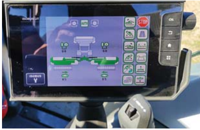
HydraForce developed a new electronic control system for the SaMASZ mower which allowed implementation of ISOBUS, providing operators with the ability to choose all of the implements' functions from a virtual terminal leading to improved ease of use.
