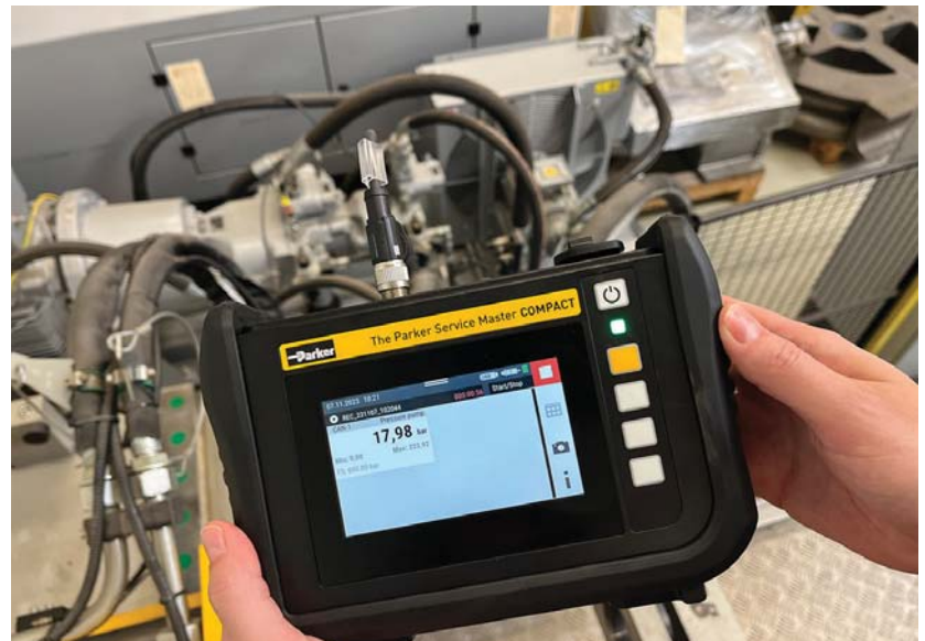
The SensoControl handheld device from Parker Hannifin’s Quick Coupling Division can help diagnose maintenance issues with hydraulic systems in mobile and industrial applications. Parker Hannifin Quick Coupling Division
