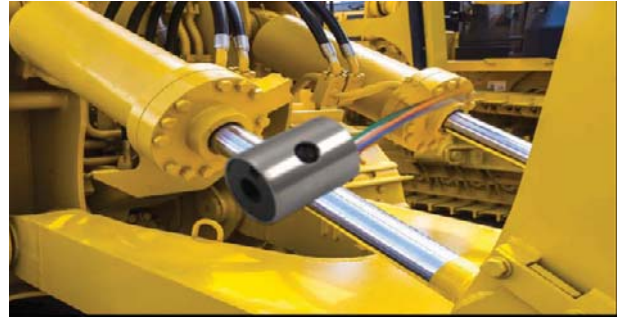
Figure 4: Vented LVDT sensors equalize pressure inside and outside the LVDT to operate reliably in temperature extremes of -65^{\circ}\text{F} to +400^{\circ}\text{F} and operating pressures of 30,000 psi. Offering a lightweight, low-mass core and a compact 3/8-in. diameter, these miniature AC-operated position sensors are ideal for high-response dynamic measurement.
