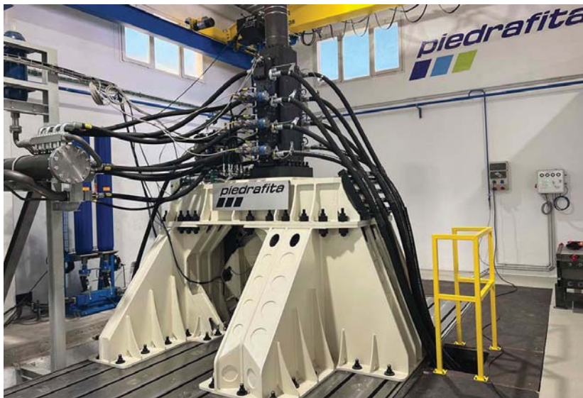
A custom-designed test bench developed by Moog and Piedrafita Systems simulates the movement of a hydraulic vehicle's tracks over uneven terrain. The system incorporates hydraulic actuators with digital servo valves, a test controller, power cabinet, digital pumps and an accumulator bench with piping. Moog
