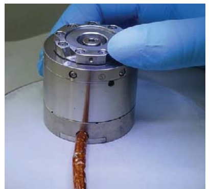
Custom two-axis, piezo-driven fast steering mirror mount for the Solar Orbiter satellite is pictured here.
