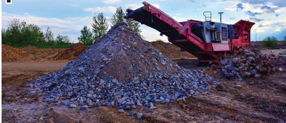
Figure 1: A jaw crusher is an essential part of operations at many quarry sites, using compressive force to break down large pieces of material into smaller, more manageable parts. Images courtesy Fleming Controls and Power Specialties, Inc.
