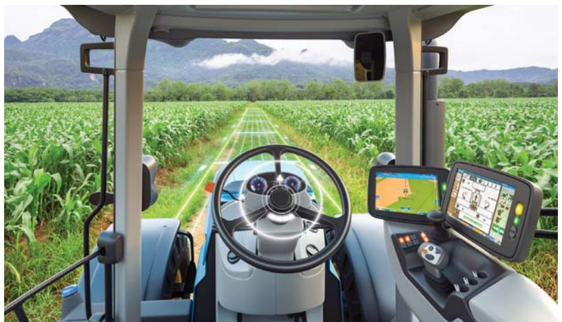
With Level 2 autonomy, operators are still responsible for directing and monitoring operations, but certain machine functions, such as steering, can be automated.
