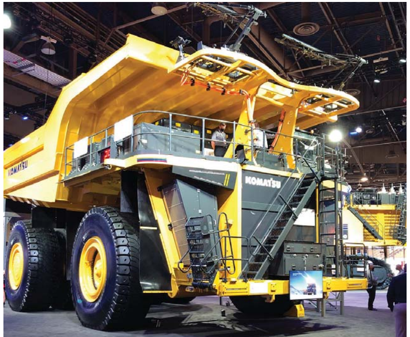
Use of overhead catenary wires, also referred to as trolley systems, allow electric mining vehicles to charge continuously during operation. S. Jensen
