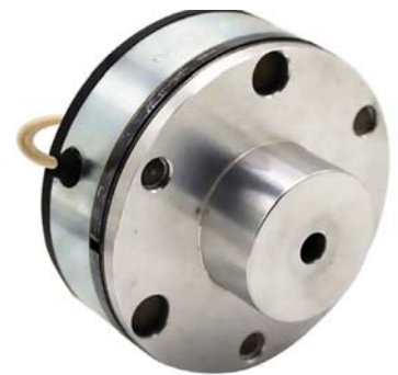
Permanent magnet brakes, like the one shown here, use independent permanent magnets to counteract and oppose the magnet flux generated when power is supplied to the coil of the brake.
