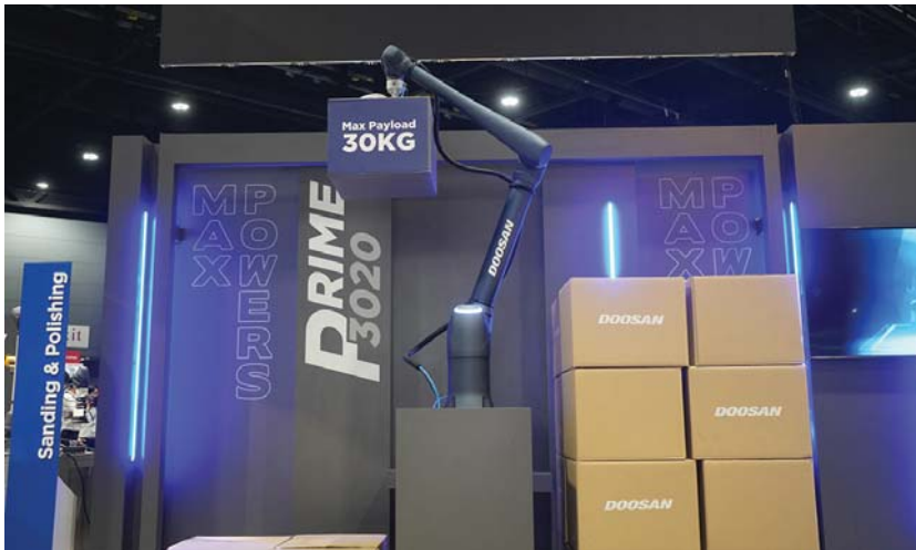
Doosan also unveiled its P3020 cobot at the show. The cobot has a payload of 60 lb and can palletize up to two meters high without a lift. Doosan Robotics
