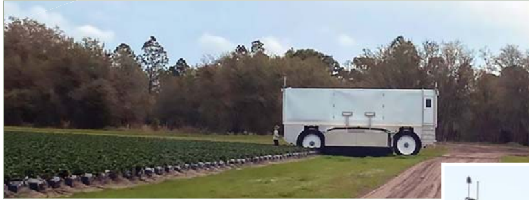
(Left:) Unlike traditional six-axis robots confined to specific tasks in controlled environments, the robotic harvester faces the complexities of delicate strawberry picking amidst the vibrations of a moving platform.
