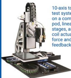
10-axis touch panel test system based on a compact hexapod, linear motor stages, and a voice coil actuator with force and position feedback
