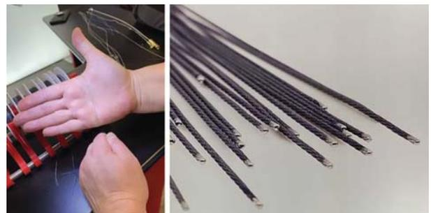
Hundreds of tungsten filaments are stranded together to create the tiny cables that are critical for making the end effectors in robot-assisted surgery work. *Sharon Spielman*
