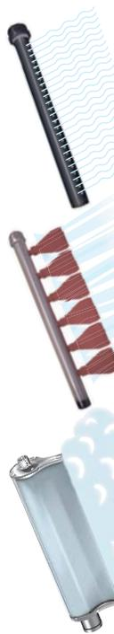
**Drilled Pipe** This common blowoff is very inexpensive and easy to make. For this test, we used (2) drilled pipes, each with (25) 1/16" diameter holes on 1/2" centers. The drilled pipe performed poorly. The initial cost of the drilled pipe is overshadowed by its high energy use. The holes are easily blocked and the noise level is excessive. Velocity across the entire length was very inconsistent with spikes of air and numerous dead spots.
