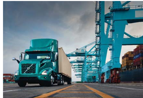
The VNR Electric is a battery-electric Class 8 truck available in North America, and among the many examples of the Volvo Group's developments in the electrification space. VOLVO TRUCKS NORTH AMERICA
