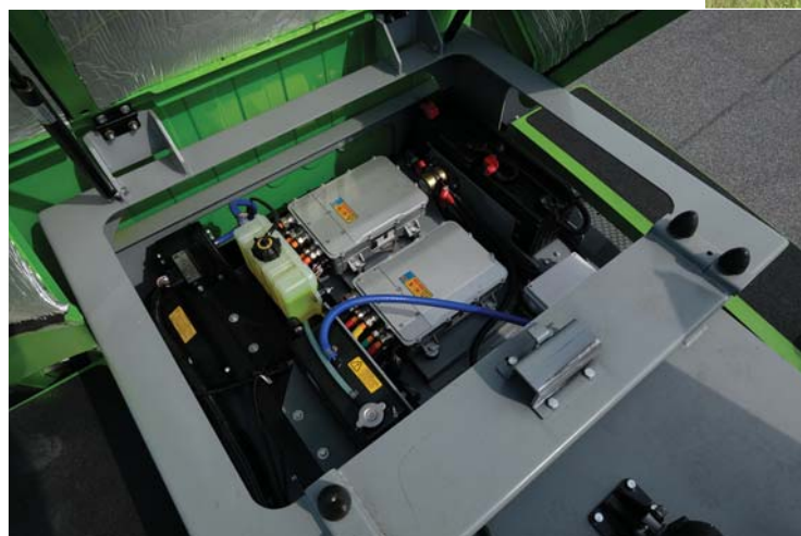
HEVI's GEL-5000 electric wheel loader is powered by a 282 kW, 660V battery which is placed at the back of the machine. HEVI
