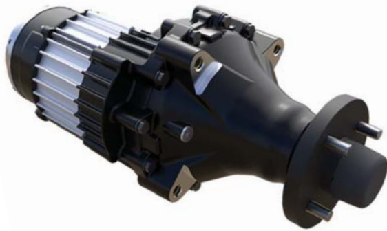
The HGMe is an electrified version of Hydro-Gear's HGM hydraulic wheel motor which utilizes the same hydraulic geartrain but with a brushless DC motor attached. HYDRO-GEAR
