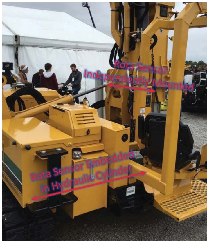
Two different Rota position sensors were embedded with hydraulic cylinders on the Vermeer PD10 to help accurately align the machine's pile driver. ROTA LTD.
