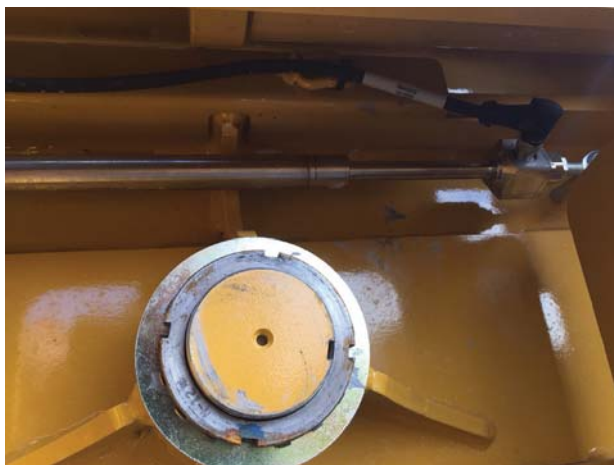
An independent mount version of the Rota position sensor was mounted in parallel to the hydraulic cylinder used with the mast of the Vermeer pile driver to keep its necessary wire harnesses safe from damage.
