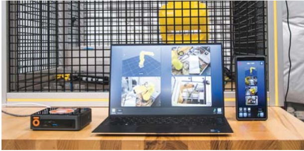
Olis Connect is controlled directly in a web browser and delivered on an Edge-hosted PC. It runs on both new and legacy automation.
