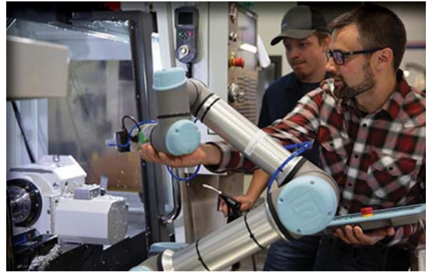
Programming a cobot for a machine-tending application. Courtesy Universal Robots
