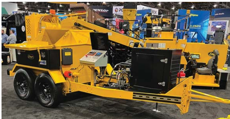
Etnyre chose to integrate the Cyclone Hydraulic Reservoir in one of its tow-behind machines, shown here at CONEXPO 2023, to help simplify the design and reduce weight.
