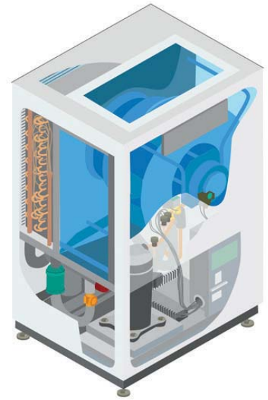
For heat pumps to operate properly, their program logic controller (PLC) needs temperature sensor inputs from multiple locations throughout the system.
