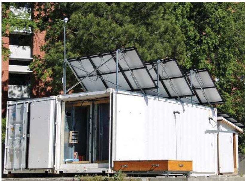
A 60-sq.-ft. chamber inside a shipping container can test passive systems that use wind towers along with water evaporation instead of electricity to cool spaces. Washington State University
