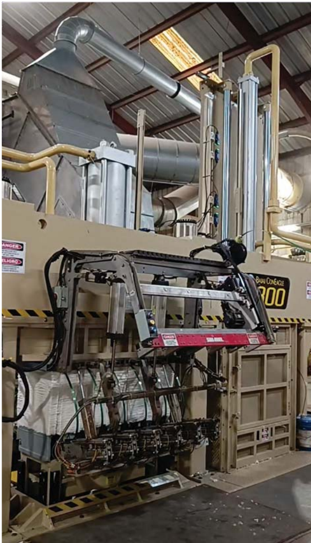
1. A cotton press with bale nearly bundled. Compressing the 480-lb bales requires significant tonnage and complex controls to ensure the machine output is consistent. Images courtesy Design Automated Controls
