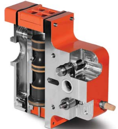
AODD pumps feature a simple, two-diaphragm design which uses a common shaft and two inlet and two outlet ball valves, suiting their use for industrial liquid-handling applications.
