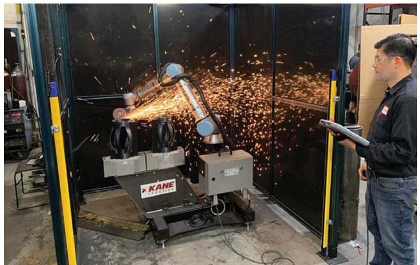
Kane Robotics’ GRIT ST cobot grinding metal industrial parts. Kane Robotics
