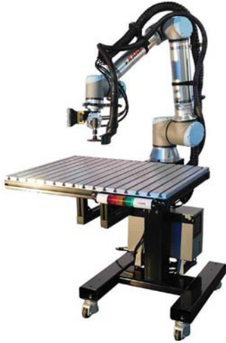
Kane Robotics' GRIT ST collaborative robot solution for sanding, grinding and finishing composites, metals and other parts in manufacturing operations.. Kane Robotics
