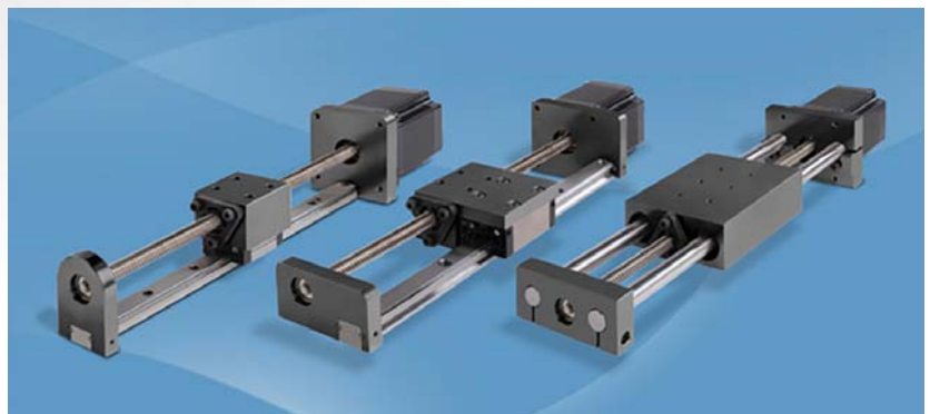
1. Standard compact linear system configurations may include the lead screw mounted vertically above profile rail (left), alongside profile rail (middle) or flanked horizontally by round rails (right). Photos courtesy Thomson Industries, Inc.
