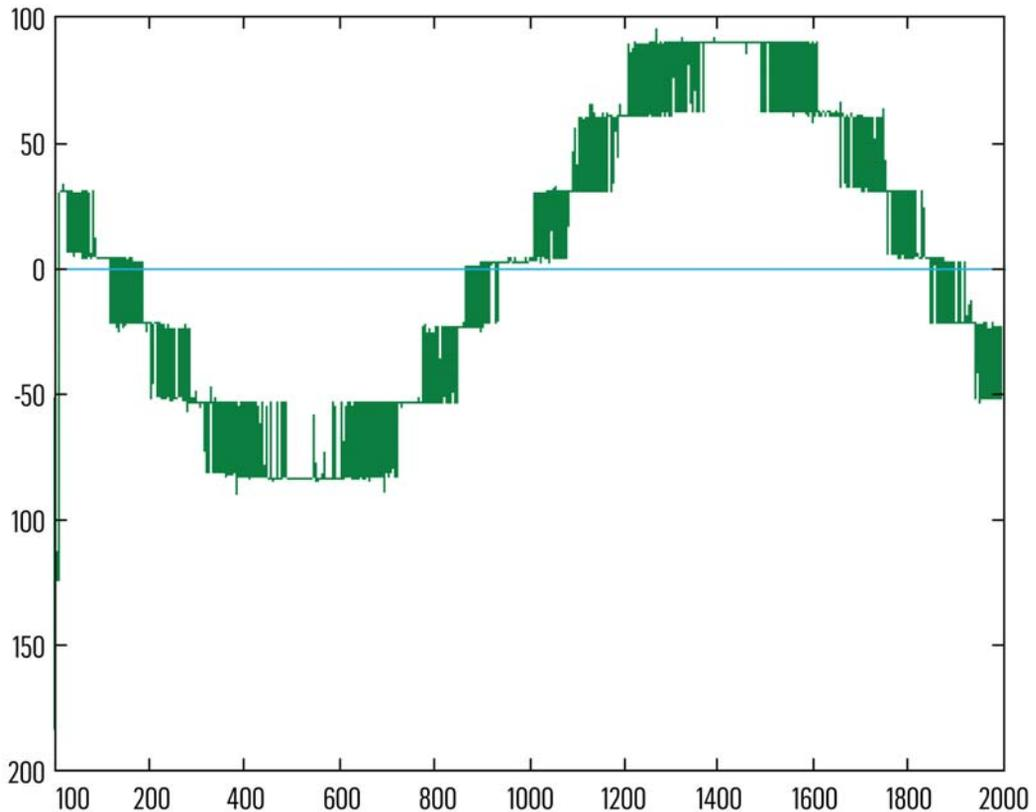
Unfiltered output from seven-level sine wave inverter (single phase).
