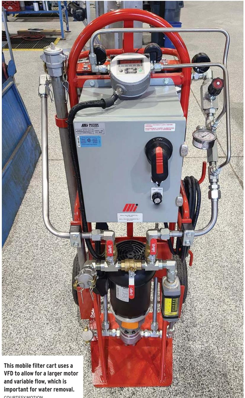
**This mobile filter cart uses a VFD to allow for a larger motor and variable flow, which is important for water removal.**
