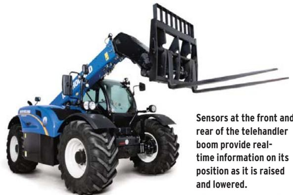
Sensors at the front and rear of the telehandler boom provide real-time information on its position as it is raised and lowered.
