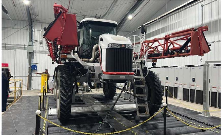
A range of construction, agricultural and other heavy-duty machinery can be tested on the new dynamometer.
