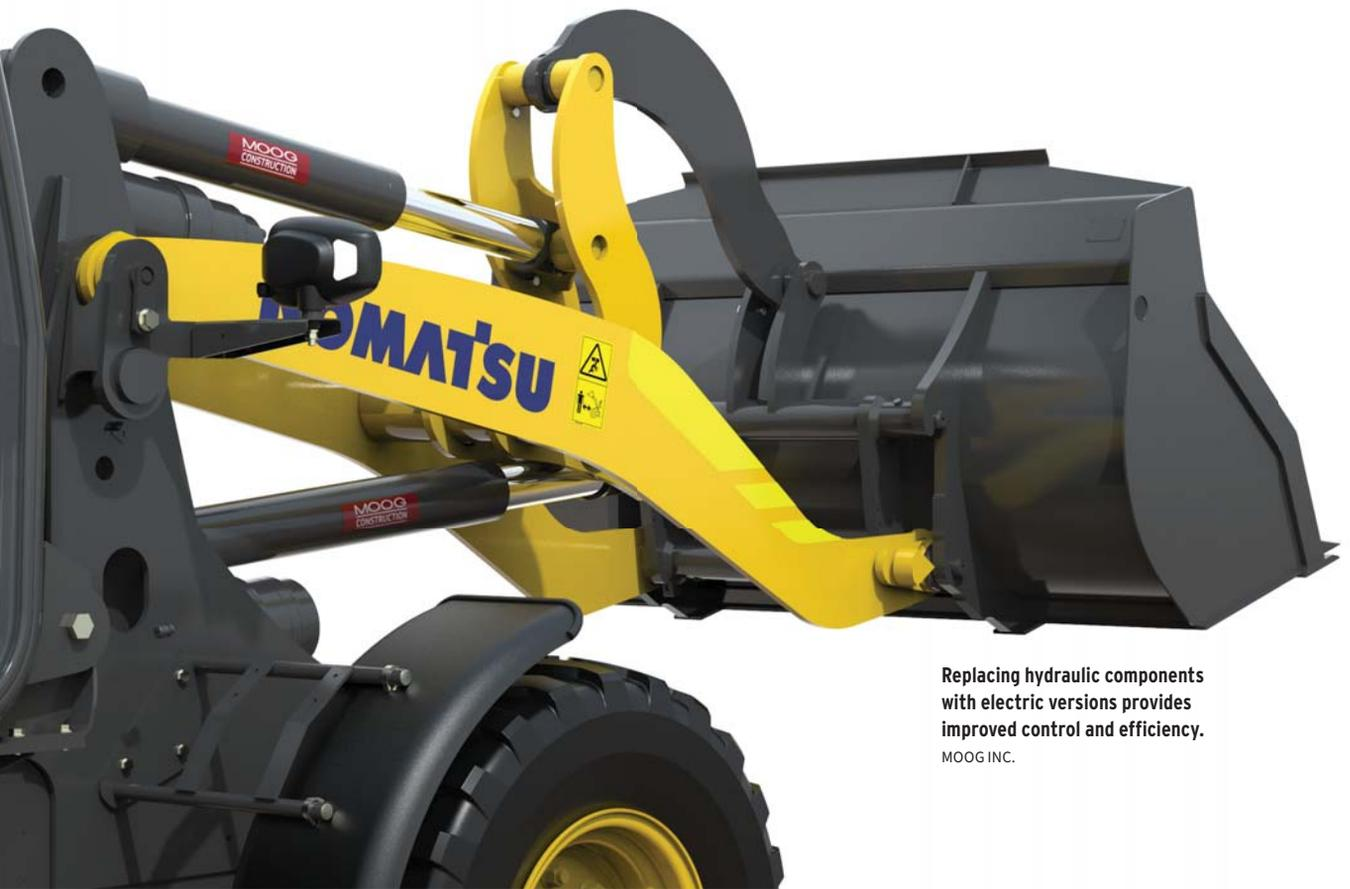
Replacing hydraulic components with electric versions provides improved control and efficiency. MOOG INC.
