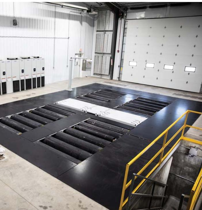
The new dynamometer at Iowa State is capable of testing wheeled or tracked machines ranging from 50-600 hp.
