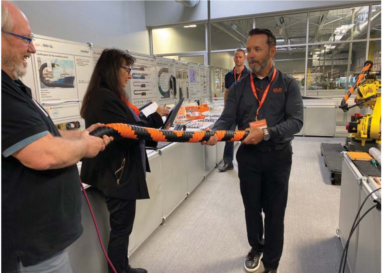
Not unlike other igus triflex R e-chains, TRX is flexible and features torsion resistance. It can be lengthened and shortened and it is also capable of 3D movement.
