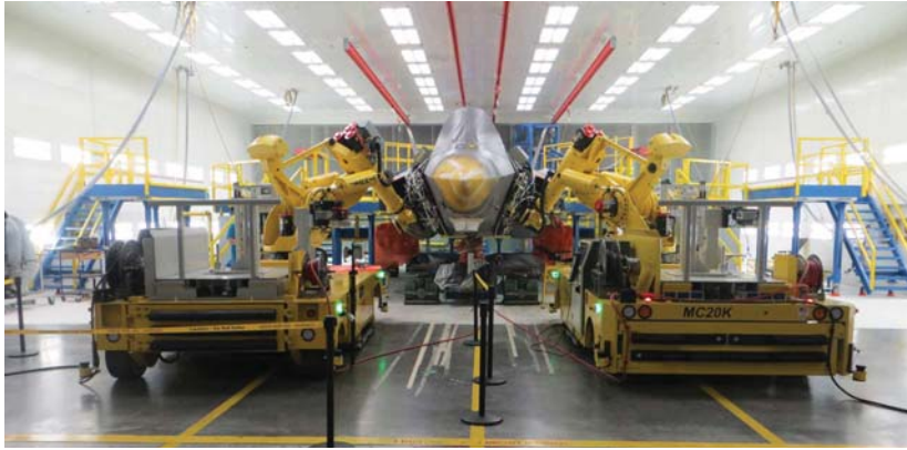
An Aerobotix robots similar to the ones used on the F-22 carry out maintenance on an F-35 using a process called Mold In Place (MIP). Courtesy Aerobotix
