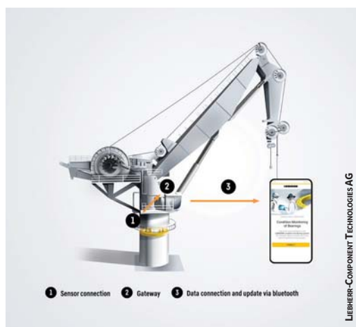
The bearing clearance monitoring system uses an integrated sensor to monitor wear as well as directions and clearance of bearings in heavy equipment. Information is stored and accessible via a mobile app.
