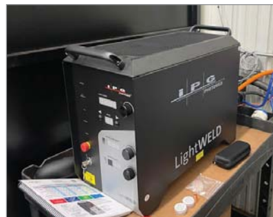
The laser-based IPG LightWELD is four times faster than traditional TIG welding.
