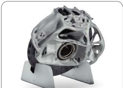
This brake assembly chassis structure, along with over 350 other components, was designed entirely by artificial intelligence and produced by laser-beam powder-bed-fusion. The mass has been reduced by over 25% for many of the components that were already designed for higher end, lightweight vehicles.
