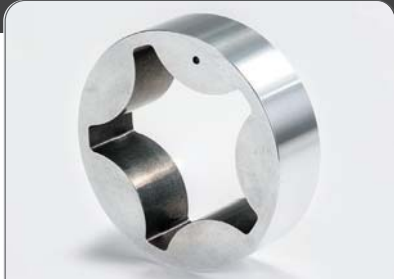
A PM aluminum outer gerotor using dual material aluminum-steel pump gears. The part provides a 50% reduction in rotating mass, which is significant, considering six gerotors per gang pump assembly.
