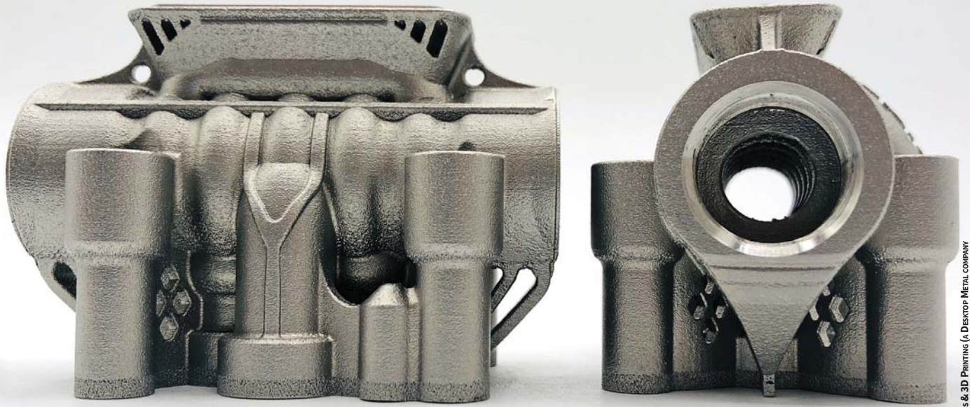
With additive manufacturing, material can be placed only where necessary, helping to reduce component weight and machining costs.
