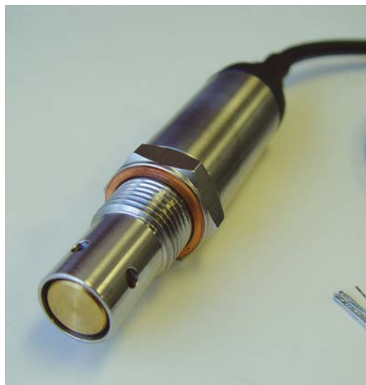
Oil condition monitoring sensor that uses the dielectric constant to determine oil condition.
