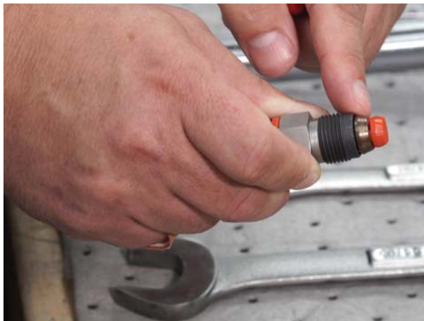
Medium-pressure mechanical grip fittings feature a preassembled cartridge that holds the two ferrules and nut, helping to ensure proper ferrule orientation during installation.
