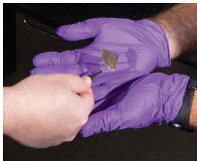
A close-up of the array of record-breaking gallium nitride diodes created by a team of Sandia National Laboratories scientists. These diodes are a step on the path to protecting the electrical grid from EMPs. Image: Rebecca Gustaf
