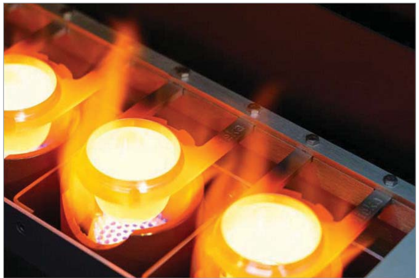
The crucible clips can be seen holding platinum crucibles over gas burners in one of Nieka's sample-making machines. The clip's design is relatively simple. But it took the company several DFMA steps to get to the final design.
