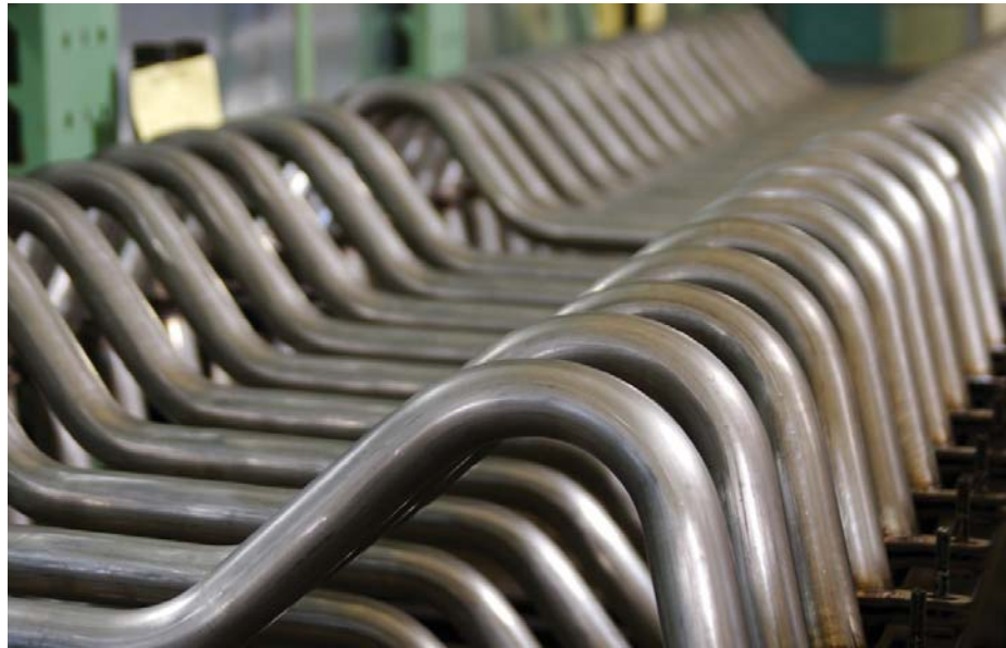
The key to running accurate, consistent metal tube bending is to correctly orient the weld seam at the outset. Sharpe Products
