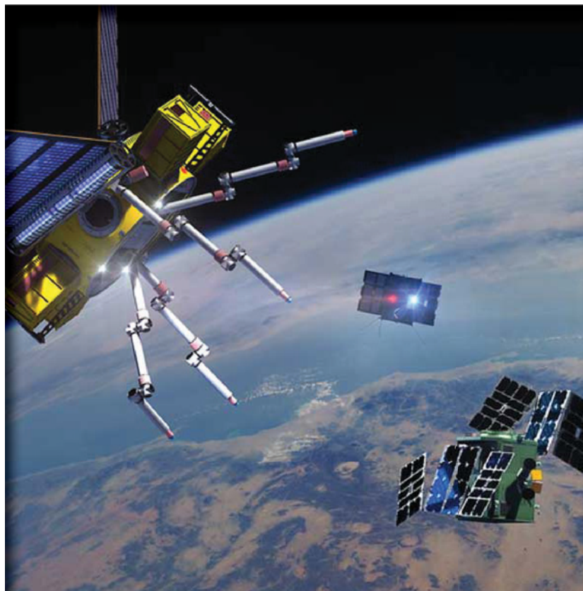
Fred, a 325-kilogram robot, will have four robotic arms. The orbot resembles a hornet, and is designed to move satellites and other objects to and from different orbits. Rogue Space Systems Corp.
