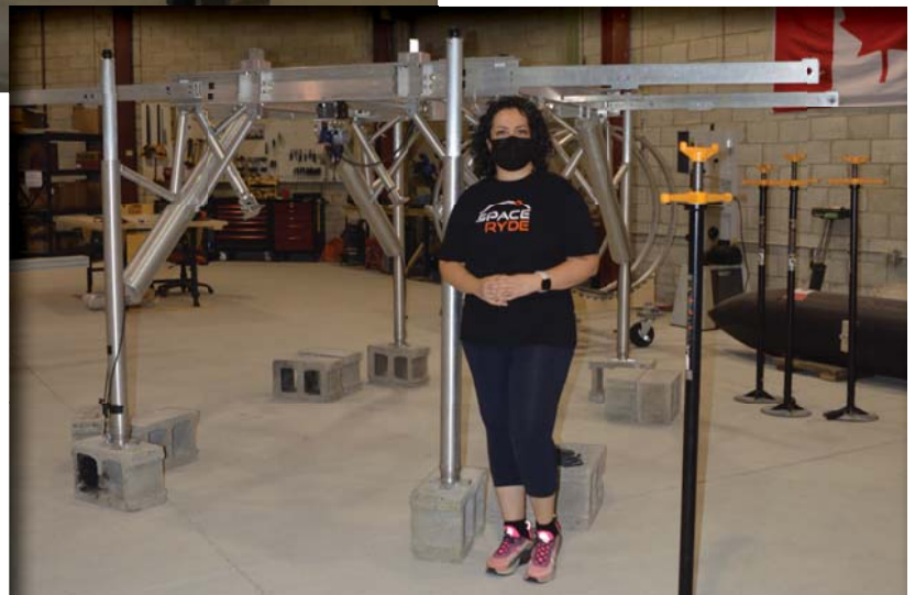
Saharnaz Safari, co-founder and COO, SpaceRyde, explained that the rocket carrier, called Flying Spider, was constructed from aluminum. This is only the second version of the design and can accommodate rockets with payloads of up to 150 kg.
