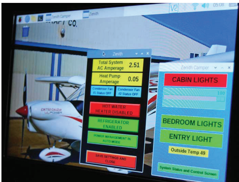
A touchscreen, operated by a Raspberry Pi, interacts with the AutomationDirect BRX PLC to provide HMI functionality for system status information and control options.
