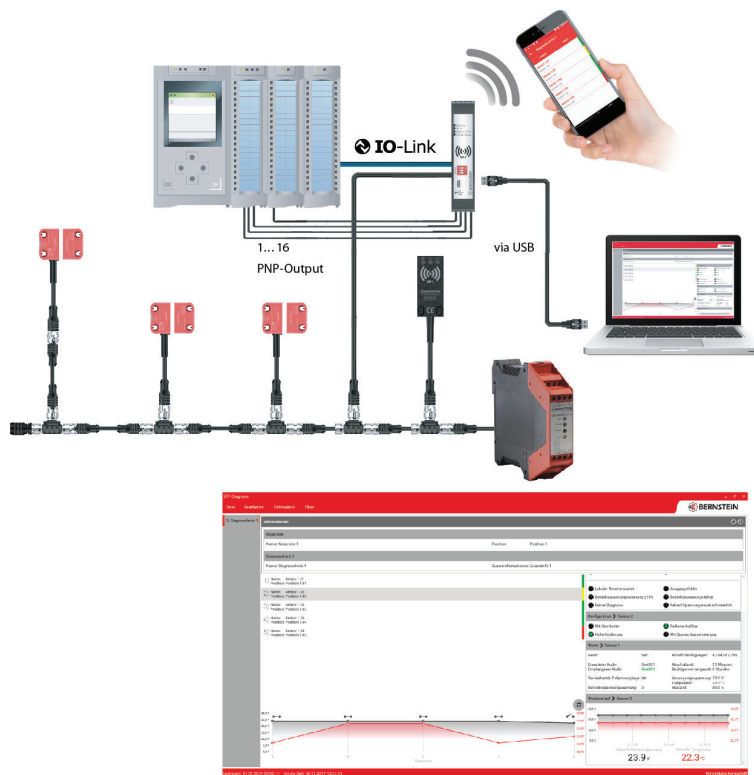
Figure 6: Safety diagnostics operate independently of the safety outputs.
