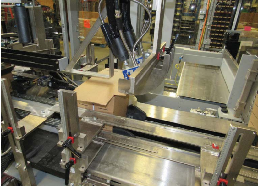
A Festo EGC for the Y axis and the ELCC for the Z-axis move the gluing system over the case flaps. Brenton Engineering
