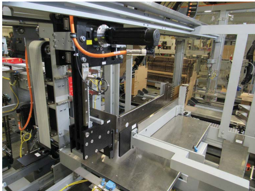
This cantilevered Y and Z axes system, center, pushes product into the wraparound case at the end of the slot. Brenton Engineering
