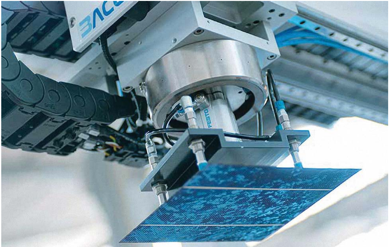
Suction-cup grippers hold a solar wafer as its moved from one manufacturing process to another.
