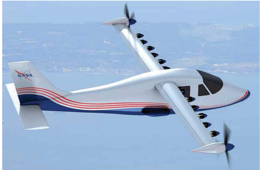
The Maxwell X-57 was one of NASA's first all-electric aircraft. It was developed to show that an all-electric airplane can be more efficient, quieter and more environmentally friendly than planes powered by gas piston engines. It uses 14 motors arrayed along the main wing's leading edge, each turning its own propeller. They are powered by a 460 V battery.
