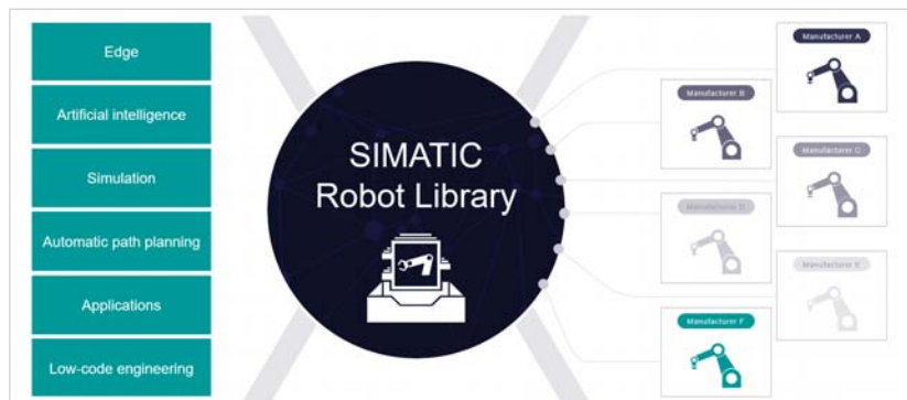
4. The Siemens SIMATIC Robot Library empowers automation programmers to control robots within a single PLC using identical programming blocks regardless of robot manufacturer. Siemens
