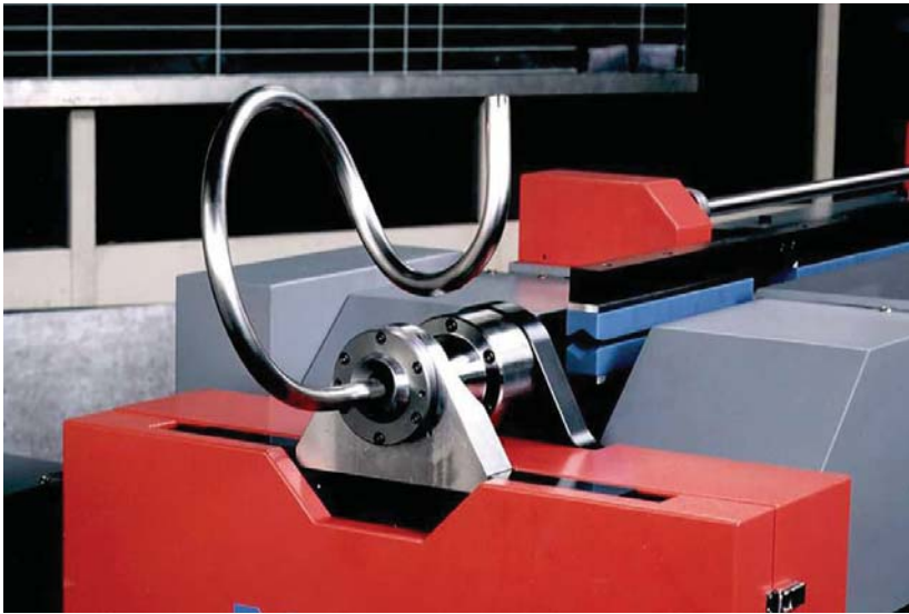
With freeform bending, the material is continuously guided through the machine using one die that is the size of the pipe or tube being bent. Nissin Precision Machines Co. Ltd.
