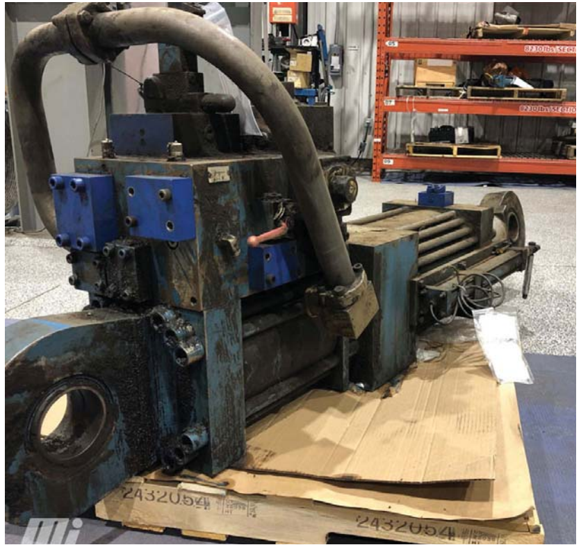
The hydraulic cylinder from the opposite page is shown before undergoing refurbishing by the Motion service center.
