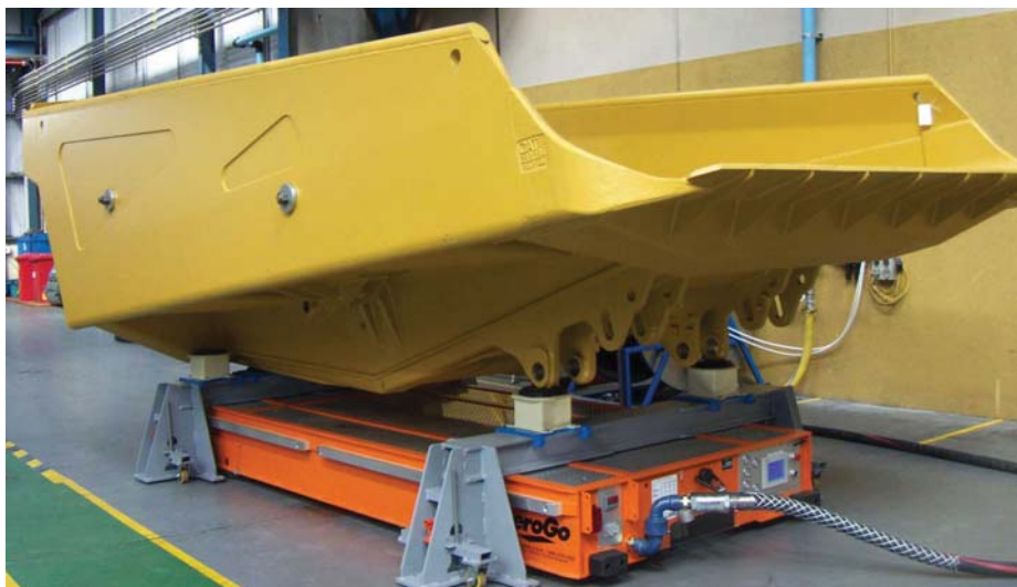
AeroGo builds remote controlled transports (orange) that utilize airbags/air casters for moving heavy loads.
