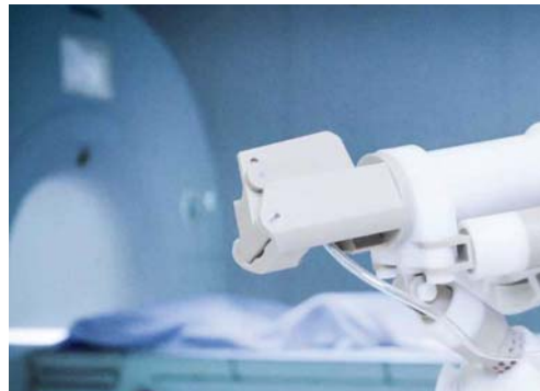
The RCM robot system from Soteria Medical is used inside MRI machines to take biopsies of tumor tissue in a patient's prostate gland. To make the robot free of any metal that would disturb the MRI machine, it uses pneumatic actuators and controls from Festo.
