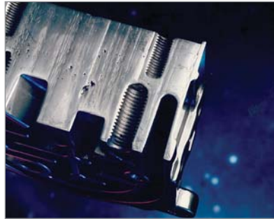
Porosity is a recognized issue with die-cast components. Microscopic holes created within a part during casting may leave the part nonfunctional due to leaks.
