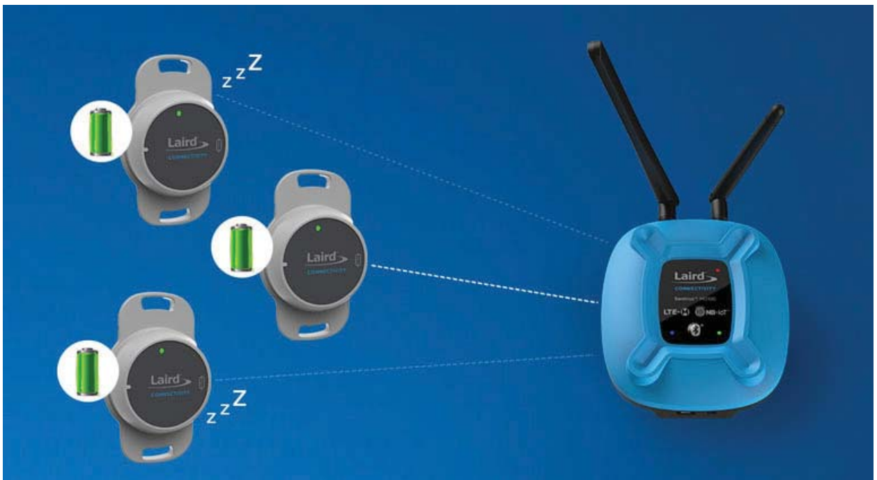
2. Ultra-low-power cellular protocols designed for low-bandwidth IoT applications use wireless devices that only need to infrequently transfer data. After those occasional data transfers, the sensor or other device can quickly go back to sleep, minimizing the drain on the battery.
