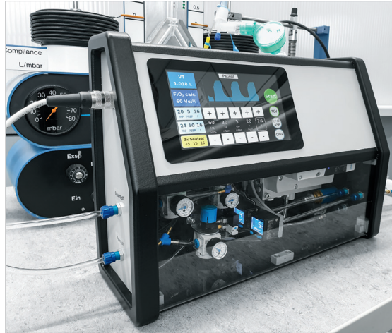
This Festo prototype for an emergency ventilator is based on piezo proportional-control-flow valves.
