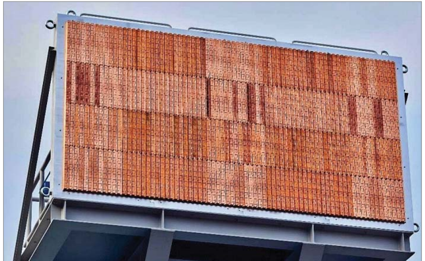
▶ 3. This 2,000-element SWAA from Mitsubishi Electric and Hiroshima Institute of Technology is designed for use in weather and surveillance radars.
