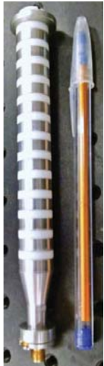
◀ 2. The omnidirectional ring-based SWAA antenna from researchers in Brazil is designed to deliver coverage indoors or outdoors with substantial gain.
