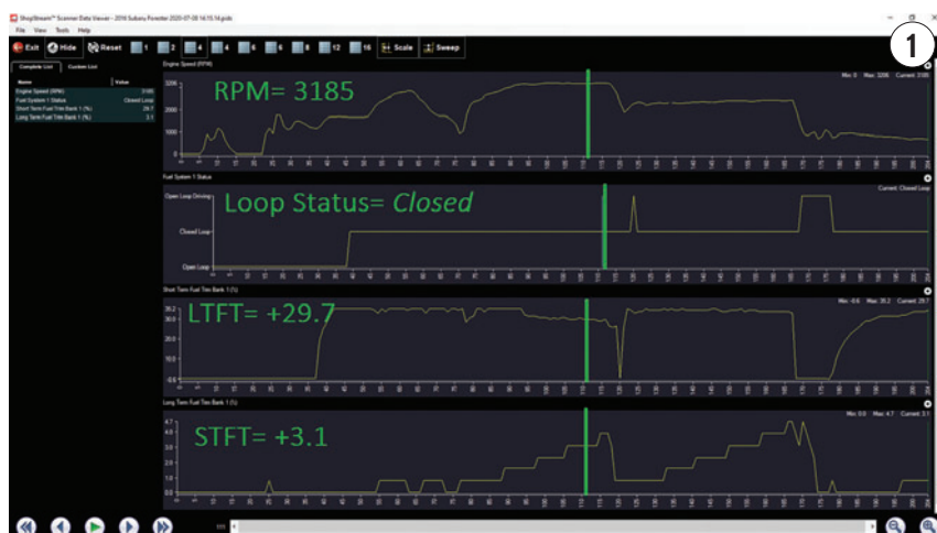
A SCAN DATA RECORDING OF A NON-FFV being driven with too much ethanol in the fuel tank.
