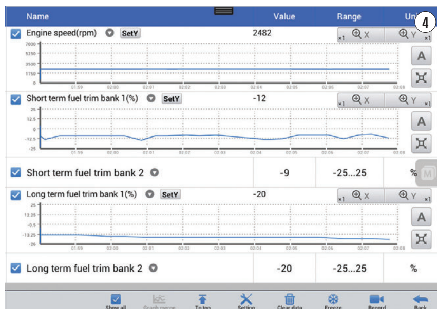
FUEL TRIMS FROM A 2011 SILVERADO with an incorrectly learned ethanol value
