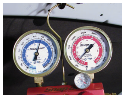
THIS GAUGE SET HAS BEEN CONNECTED TO A SYSTEM that has not been in operation. It is showing that ambient temperature is ~70 degrees and the refrigerant pressure is ~70psi. By comparing this to your chart for R-134a, this is a good indication that what is in the system is R-134a and there is enough refrigerant in the system to begin testing.
