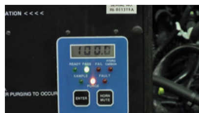
THERE ARE CHOICES FOR IDENTIFIERS. This one is showing that the system has 100 percent R-134a in it. This machine does not tell you whether the system is low or overfull, simply what is in it.
