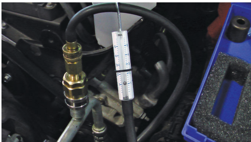
THIS VEHICLE HAS SEALANT IN THE SYSTEM. The initial starting point for this test was the band at 2.4 on the scale. After 90 seconds, the flow has dropped to 1.0 indicating sealant in the system.
