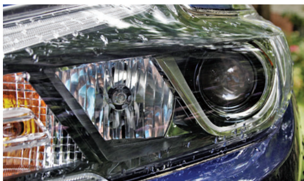
THIS 2018 NISSAN MAXIMA USES OLD AND NEW LIGHTING TECHNOLOGY. The low beams have a modern projector headlight (right) and the high beam uses a reflector, a component that's been around for more than 100 years. Both beams use halogen bulbs.
