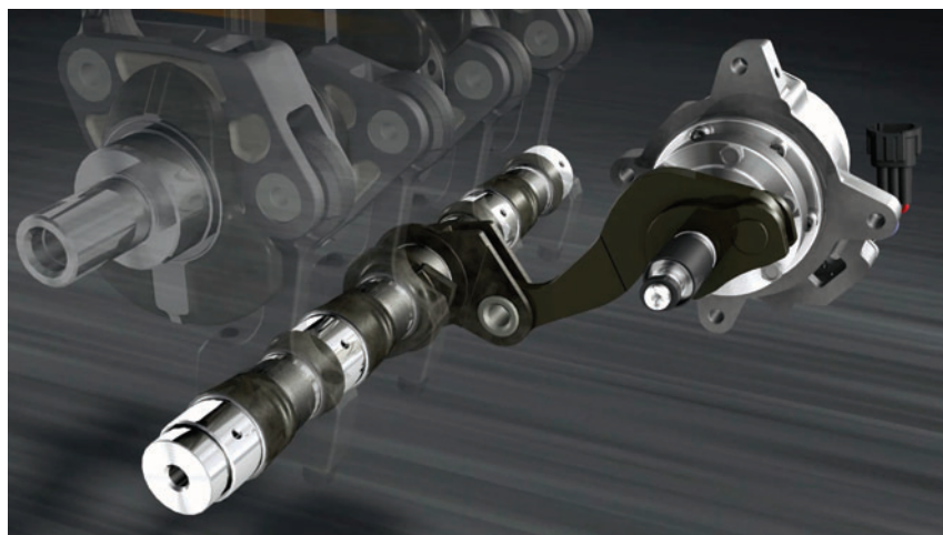
A VISUAL OF THE SHAFT UTILIZED to alter the height of piston travel via an electric motor and ECM input.
