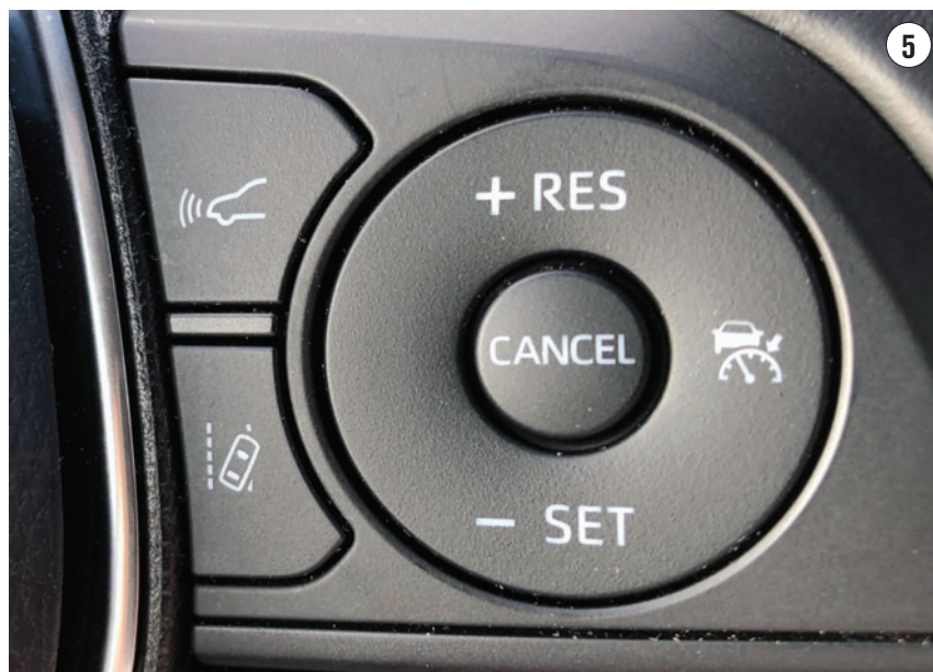
THE SWC (STEERING WHEEL CONTROL) BUTTONS ON THIS 2020 TOYOTA CAMRY use the typical "On" (far right), Set/Tap Down (bottom right) and Tap Up/Resume (top right) arrangement of switches in a circular rocker switch. The "Gap Switch" (upper left) allows the driver to adjust the distance following the next vehicle in front of them when the adaptive (radar) cruise control is in use.
