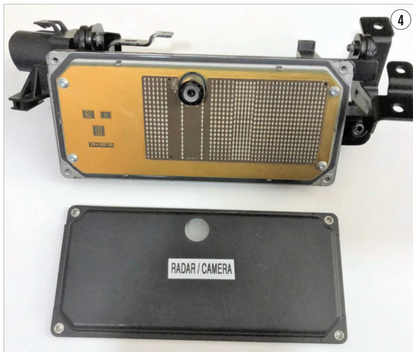
ON ADAS EQUIPPED VEHICLES, BRAKE-BY-WIRE SYSTEMS are activated by CAN bus messages initiated by software interpretations of approaching vehicles/obstacles thanks to radar sensors and cameras. This Volvo RACAM module contains both a camera (round lens in upper center of unit) as well as a millimeter electronic scanning long range radar sensor (right 2/3 of unit) to detect other vehicles, lane markings and even interpret road signs as well as establish the range of other vehicles/pedestrians.
