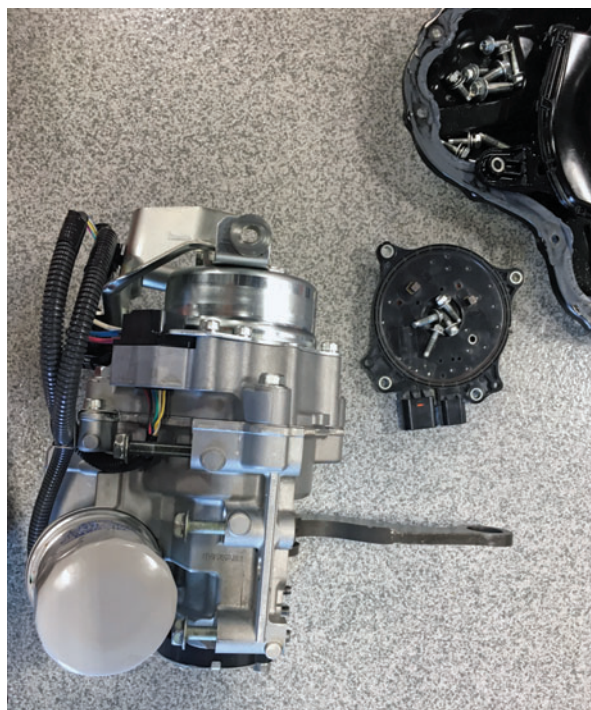
THIS MOTOR IS RESPONSIBLE FOR THE ACTUATION of the change in piston TDC height, resulting in variable compression ratios.
