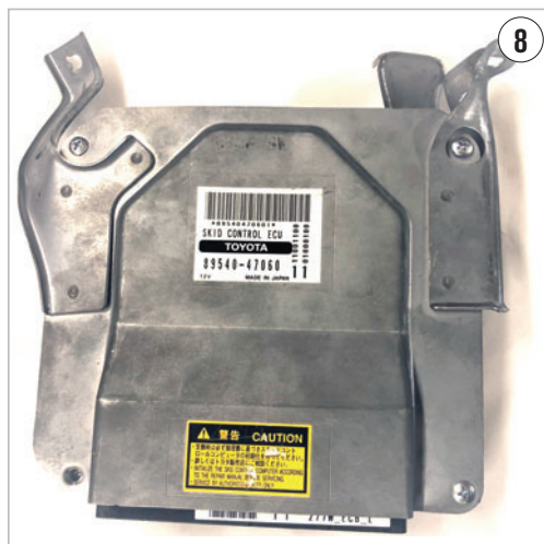
EARLIER TOYOTA HEV (HYBRID ELECTRIC VEHICLE) models (such as Prius) used a remote mounted skid control module.
