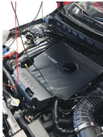
THE VC-TURBO IS A UNIQUE COMBINATION of variable compression, turbo, direct injection and other technologies.
