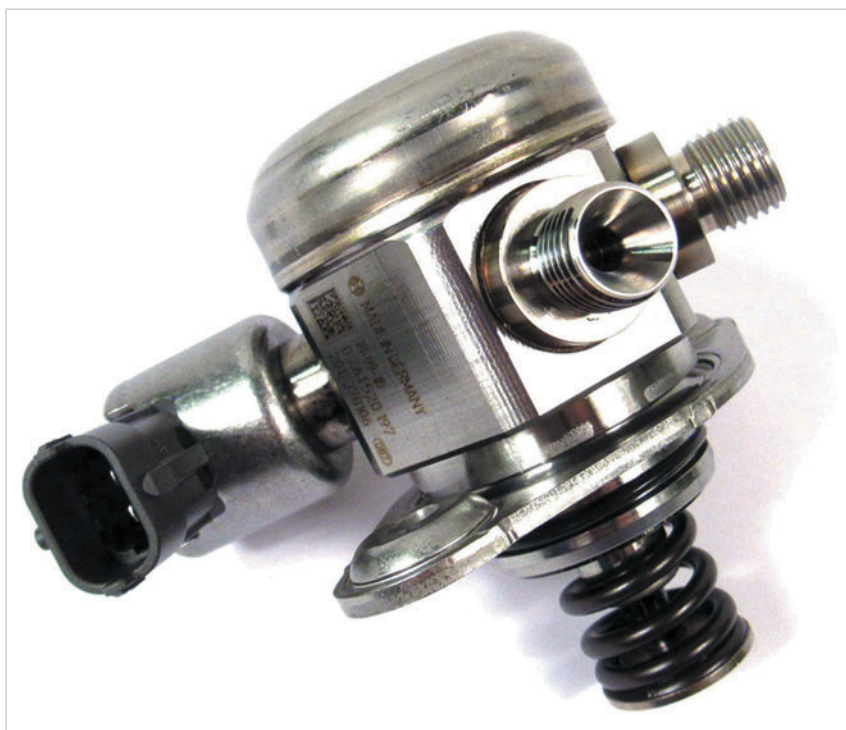
THE HEART OF THE FUEL DELIVERY SYSTEM is the high-pressure mechanical pump. These pumps are capable of creating thousands of pounds of pressure, so exercise caution when servicing or repairing any of the high-pressure components.
