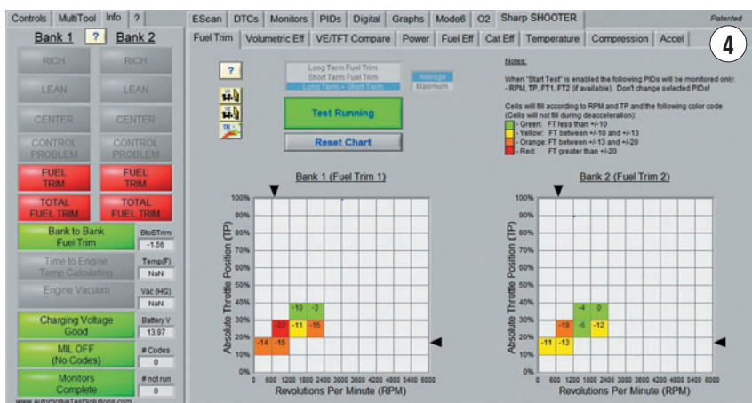
SECOND ROADTEST using escan fuel trim test captured problem.
