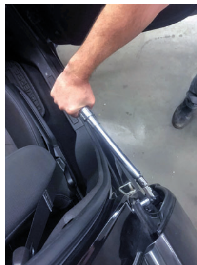
TORQUING A DOOR HINGE BOLT TO SPECIFICATION
