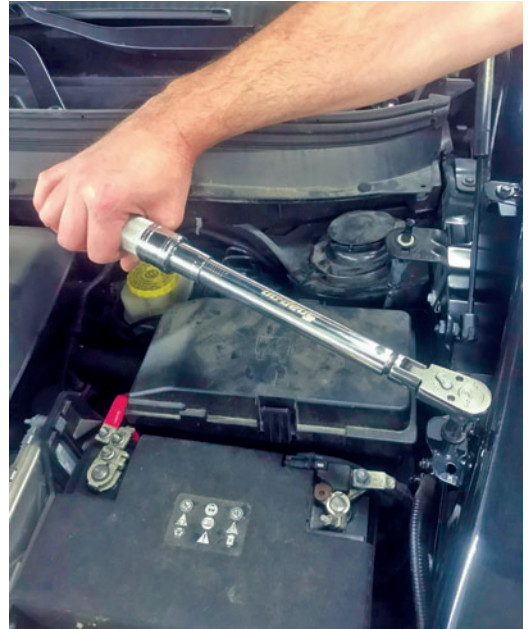
TORQUING A FENDER BOLT TO SPECIFICATION
