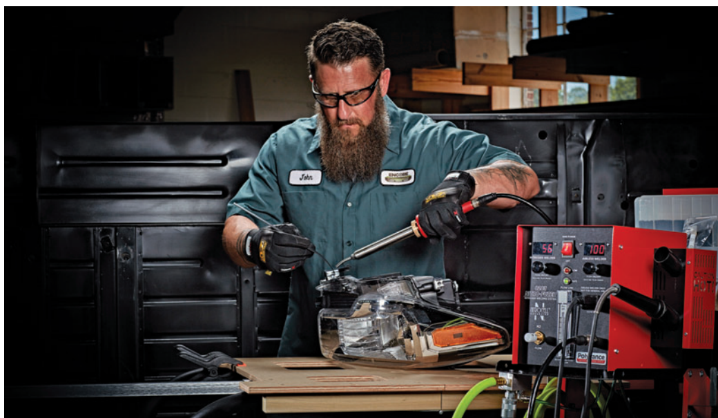
THE FIVE IMPORTANT FACTORS for plastic welding are T.F.A.P.S. (Temperature, Flow, Angle, Pressure and Speed). Make sure your equipment settings and processes follow all five.
