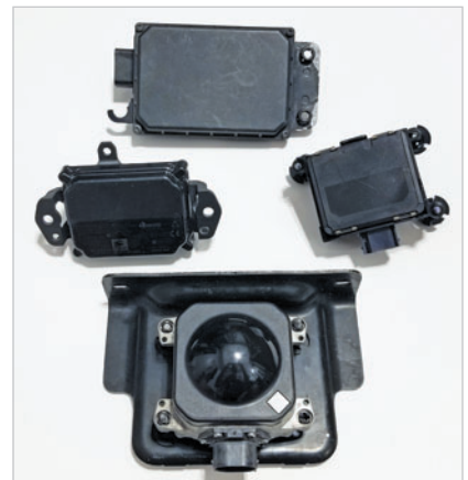
FORWARD FACING RADAR UNITS come in many shapes and sizes and are sometimes mounted behind emblems or covers.
