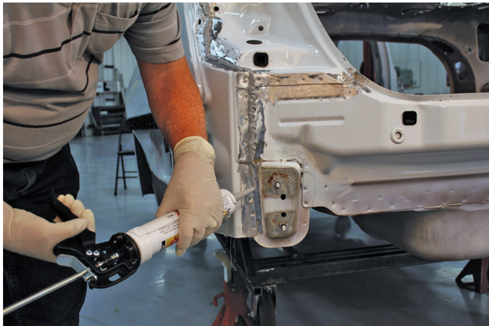
DIRECT-TO-METAL SEAM SEALERS BOND WELL TO BARE ALUMINUM AND STEEL TO PROTECT THE REPAIR AREA.
