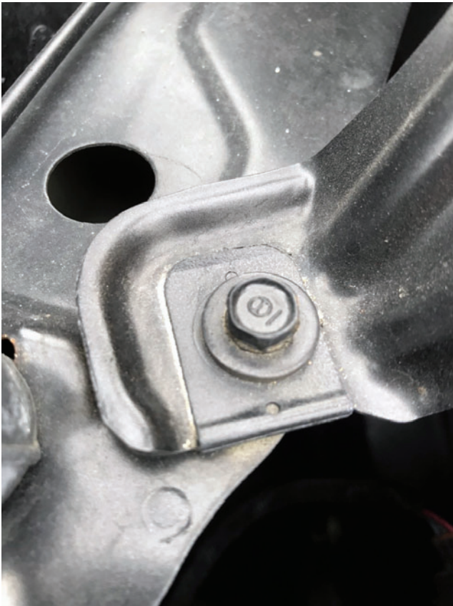
EXAMPLE OF A MANUFACTURER using a barrier between the dissimilar metals of a fastener and an outer body panel. Barrier is below the screw head.
