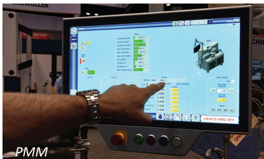
Graham Engineering’s American Kuhne-brand Compact Modular MD extruder is equipped with the XC300 Navigator control system.
