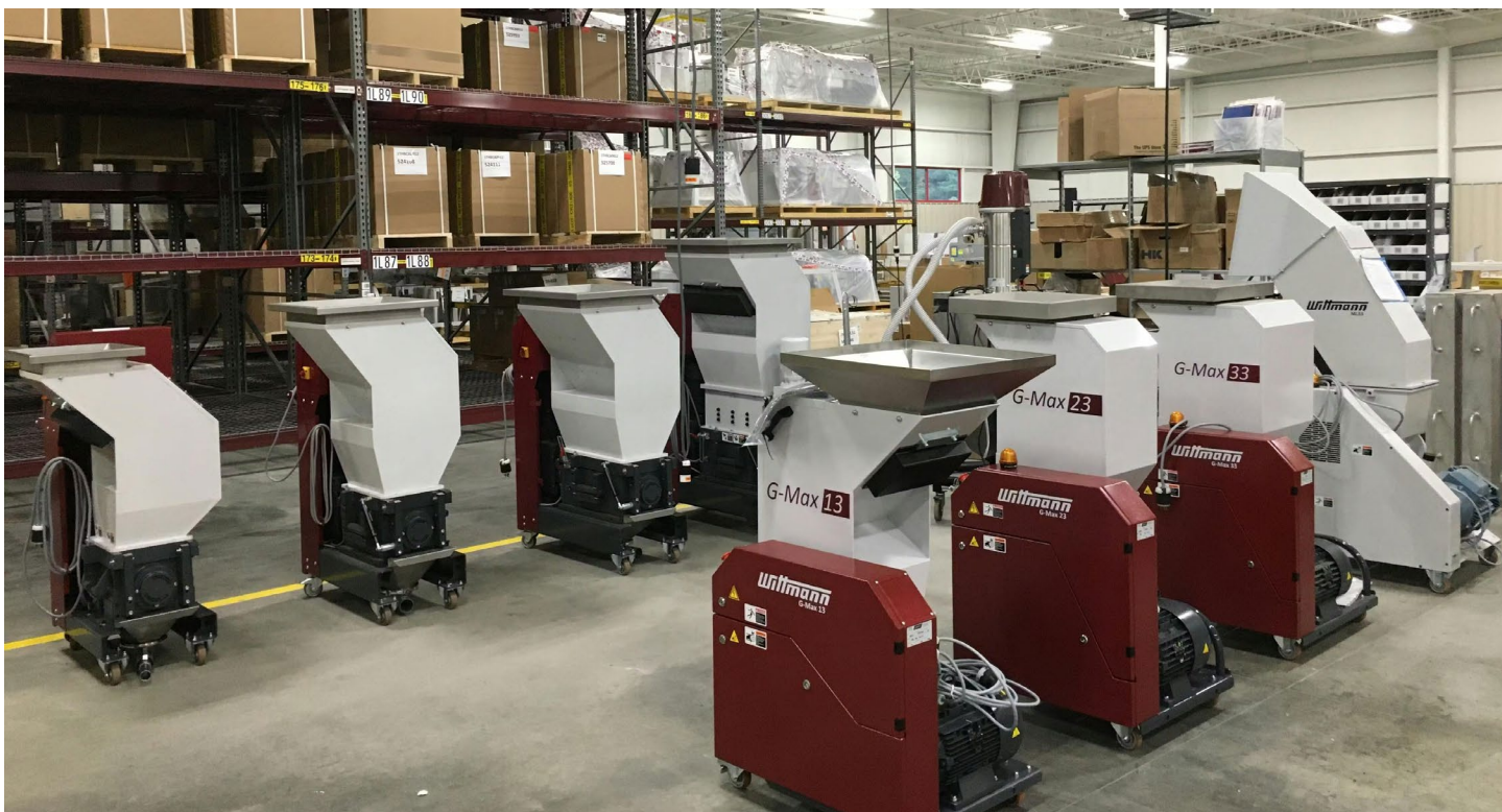
Wittmann USA's facility in Torrington, Conn., is set up with a range of granulators to test customers' materials and determine the best equipment solution. | Photo credits: Wittmann USA
